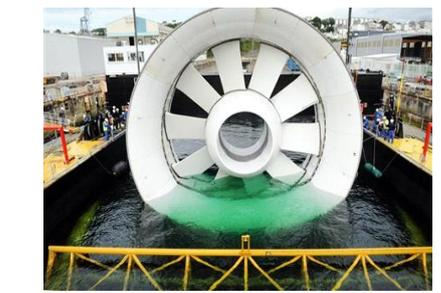
HYDROLIENNE OPEN HYDRO ASSEMBLE A DCNS BREST
